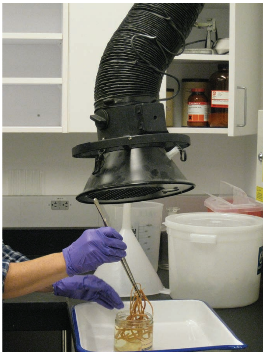
FIGURE 9.11 Fume extractor or snorkel.
